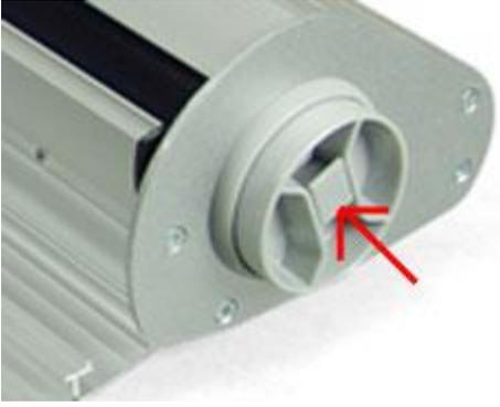
The tension release is used to release tension on the retraction spring. This is only required if the banner is to be replaced or there is a problem with the unit. **DO NOT** release tension on the spring while the banner is in the raised position. Damage to the spring and overall unit may occur. Remove the banner once tension has been released.
