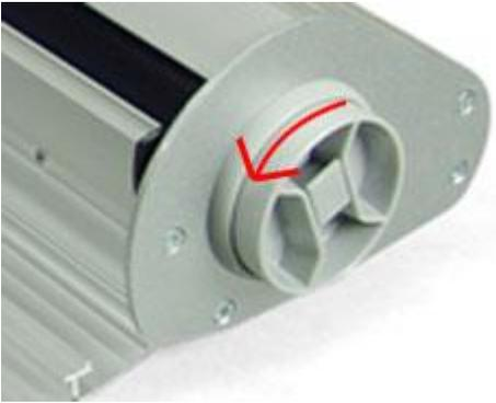
The rotating knob is used to add tension to the spring. It should only be used when replacing the banner. **Applying too much tension to the spring will damage the unit.** **Too much tension may also cause the banner to curl more than normal.** Tension on the spring will increase as the banner is raised.
