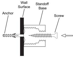
**IMPORTANT:** Check the base of each standoff is securely tightened after attaching to the wall.
