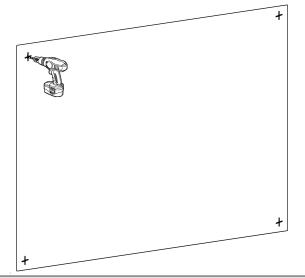
3. Separate each standoff from the base. Insert the nylon anchors into the pilot holes and tap them flush with the wall surface. Screw in the base of each standoff until they are securely fastened.
