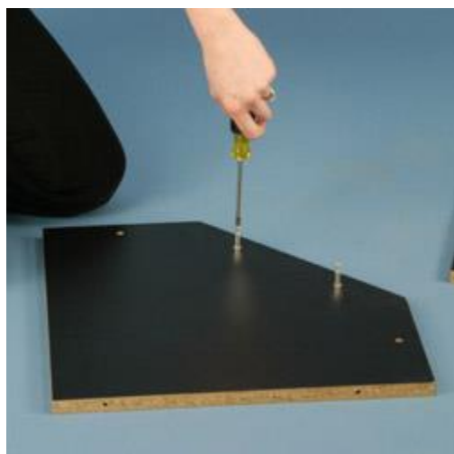
Step 1 Using a Phillips head screwdriver, screw in two bolts.
