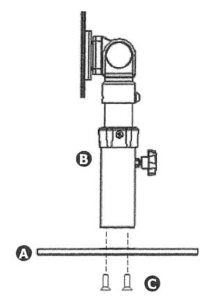
Fasten base (A) to upright (B) with provided flat head screws (C).
