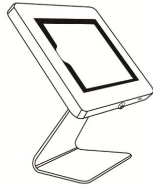
Close the Case and press the Lock Button to lock
