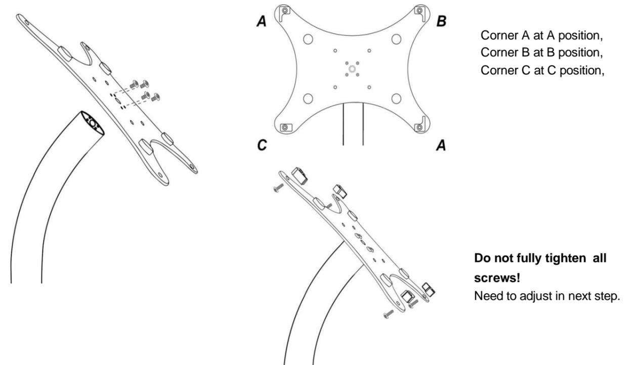
Corner A at A position, Corner B at B position, Corner C at C position,
