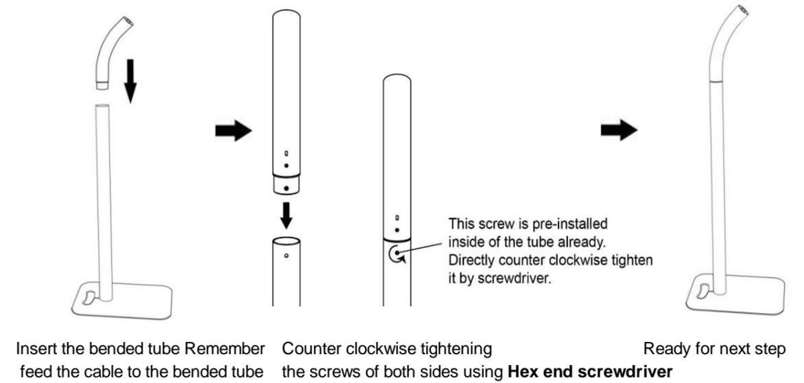
Insert the bended tube Remember feed the cable to the bended tube
