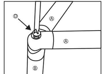
Using the short screws (D) attach the Short Bar (B) to each corner as pictured.
