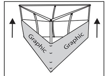
With the help of another person, position your graphic so the center seam is centered with the bottom frame and the corners are aligned. Raise the graphic up and over the outside of the frame.
