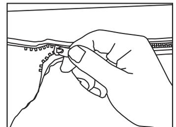
Once all long screws are in place, lift the inside of the graphic and zipper The sections together.
