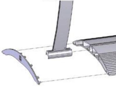
**4.** Slide the second side support into the base and secure it in place with a screwdriver. (Please remember to connect the poster bar as well.) Replace end cap.
