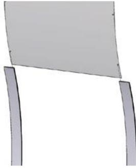
**5.** Insert poster and lenses (at the same time) into the grooved channels. Make sure the bottom portion of the poster slides into the bottom bar.
