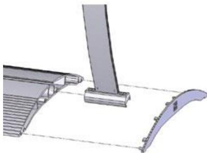
**1.** Remove end cap from base. Slide (1) side support into base and secure it in place with a screwdriver. Replace end cap.
