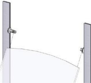
**7.** Insert each acrylic pocket into the brackets. Make sure your pocket is lying flush against the bracket to ensure a secure connection.
