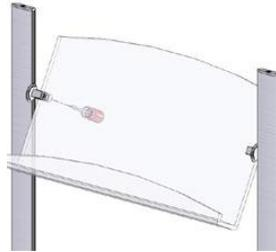
**8.** Secure your accessories in place by tightening the plastic set screws.
